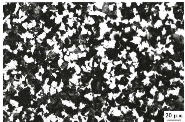
图3 工艺优化后 38CrMoAl 钢盘条组织形貌 Fig. 3 Morphology of structure of steel 38CrMoAl coil after process optimization
